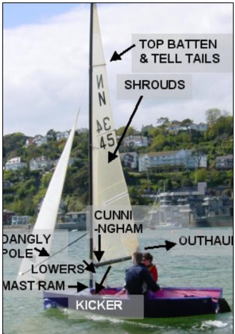
In general the following can be done to control the power in the rig at different points of sailing.
