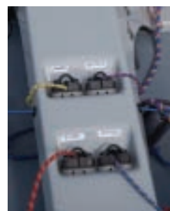
Above The rig is extremely adjustable with controls for shrouds, lowers, cunningham, kicker, mast ram and jib luff tension led to either side of the cockpit.
