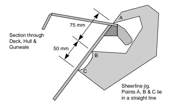
Construct jig from rigid material (e.g. 6mm perspex). Hold in a vertical plane with points B and C against side of Hull and point A resting on top surface of Deck.
