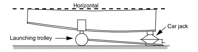
With a helper, set Sheerline points at Bow and both sides at the Stern level by sighting against water level in a tube held against them. Holding level in tube steady against Sheerline point at one end of Boat, move tube along each side of Boat to Sheerline marks on Deck. Check that all marks between Bow and Stern are below water level (i.e. below horizontal).
