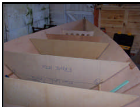
Picture (right) shows the hull with sheerline trimmed
