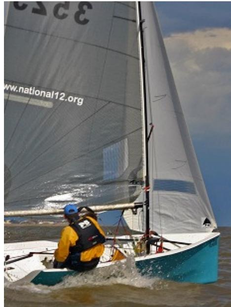
You will obviously both be sat out hard and the boat should be set up with slight lee helm (so the boat naturally bears off slightly in a gust, if the boat luffs up you will stop dead). With practice you can also use the Winged rudder upwind for more lift and speed.
