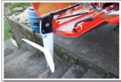
control pitching moment as well. Shown are a couple of images of retrofitted systems which differ greatly in the way they operate. Dare Barry's Pudding design has a Composite Craft built rudder and stock, with all the adjustment happening within the stock itself, making for relatively easy transfer of the system between boats. .
